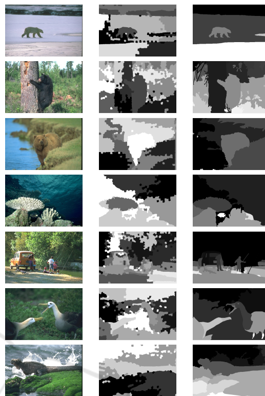
Figure 4: Exemplar segmentation results obtained by the proposed method on the BSD500. Left column: raw images; middle column: achieved segmentation; right column: ground truth segmentation.
