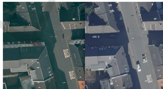
Figure 1: Orthophoto (left) vs. true orthophoto (right).
