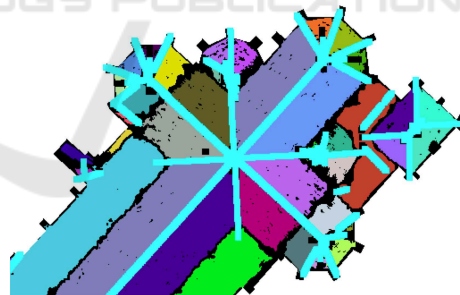
Figure 4: Intersection lines between estimated planes.
