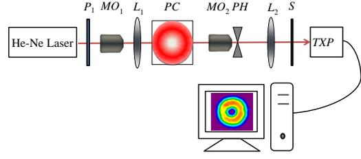
Figure 1: Proposed experimental setup.  $P$ : linear polarizers;  $MO$ : microscope objectives;  $L$ : lenses;  $PC$ : polarization converter;  $PH$ : Pinhole;  $S$ : sample;  $TXP$ : light polarimeter.
