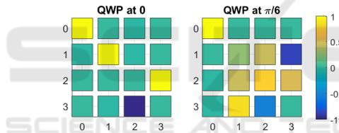
Figure 2: Experimental Mueller matrix for a QWP with its axes at 0 (left) and rotated  $\pi/6$  (right) relative to the  $x$  axis.
