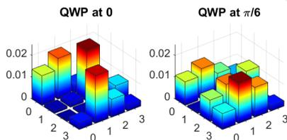
Figure 3: Absolute values of the differences between theoretical and experimental Mueller matrix elements for a QWP with its axes at 0 (left) and rotated  $\pi/6$  (right) relative to the  $x$  axis.
