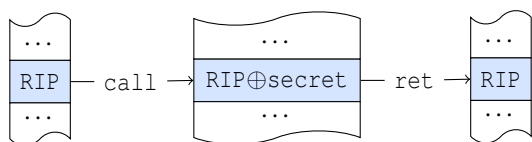
Figure 3: The XOR security module.
