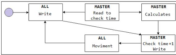
Figure 3: Webots proposed controller represented in a finite state machine to control the team of robots.
