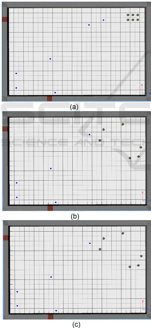
Figure 4: Simulations in Webots EDU: (a) Initial configuration. (b) Odometry without angle maintenance. (c) Odometry with angle maintenance.
