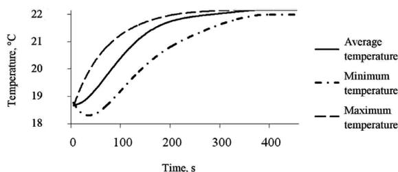
Figure 3: The graph of transient on volume in the calculation area. Initial temperature 19 °C.
