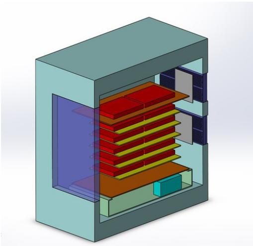
Figure 8: Cross-section of three-dimensional model of device for storage of the transfusion environments containing platelets.
