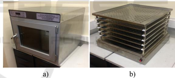
Figure 7: The appearance of intelligent storage devices for transfusion environments containing platelets. 7a) - heat insulated chamber with thermostating electronic device and control system of storage regime parameters and 7b) – presents electro mechanic module.
