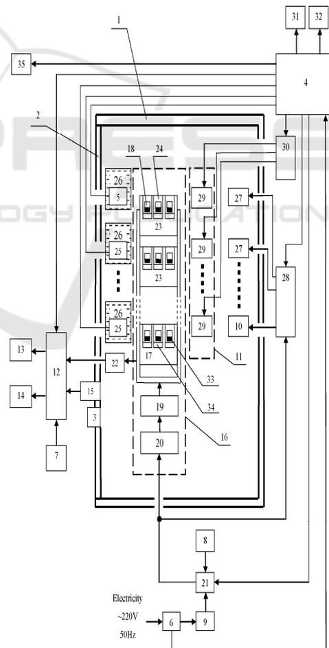
Figure 10: Structural scheme of the intelligent device for storage of the transfusion environments containing platelets.
