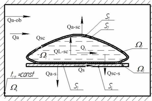
Figure 1: A design scheme for a polymeric container with transfusion environments containing platelets.
