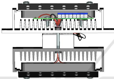
Figure 5: A computer model of the thermo battery using thermoelectric semiconductor elements (side view).
