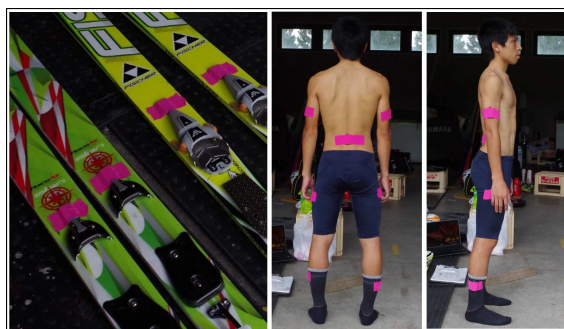
Figure 1: Nine sensors were attached to the athlete's body and ski to capture the ski jumps.
