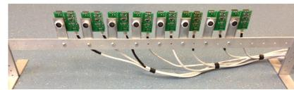
Figure 8: Physical disposition of an ultrasonic array - linear mode.
