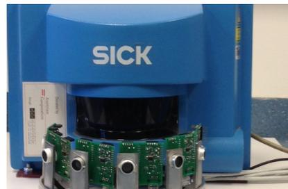
Figure 9: Physical disposition of an ultrasonic array - circular mode.
