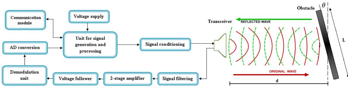
Figure 3: Ultrasonic cell structure.
