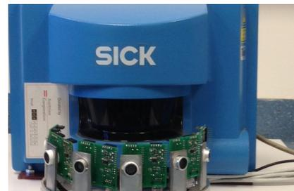
Figure 9: Physical disposition of an ultrasonic array - circular mode.
