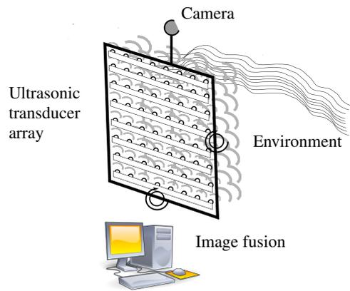
Figure 1: The hybrid 2D imaging system - ultrasonic cells and RGB camera. Sensor array is mounted on a platform with optional two degrees of freedom for an improved spatial coverage.
