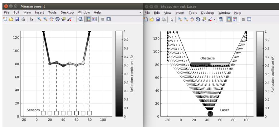
Figure 10: Left: visualisation of measurement results obtained by linearly disposed ultrasonic cells, Right: visualisation of laser measurements and presentation of the actual obstacle. Different grayscale tones are used for depicting the determined reflection coefficient.
