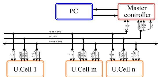
Figure 7: The topology of the distributed sensory system.
