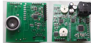
Figure 4: Physical implementation of the ultrasonic cell. The dimensions of the cell are  $5 \times 5$  [cm], with the possibility of reducing the dimensions to  $2.5 \times 5$  [cm] by cutting and stacking the two segments of the PCB on top of each other.
