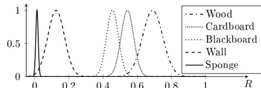
Figure 6: The dispersion of the reflection coefficient  $R$  for different materials.
