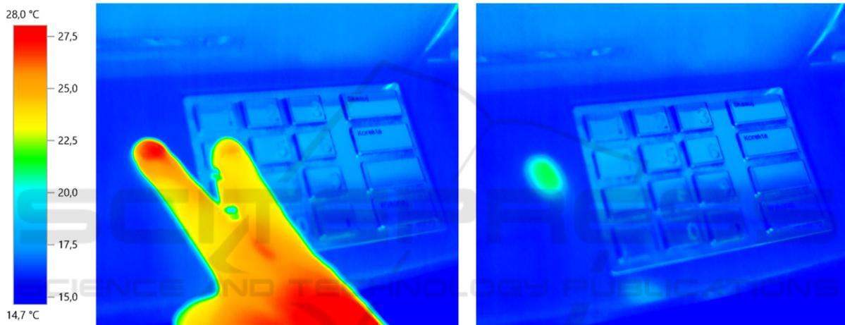
Figure 5: Attack on a cash machine (metal keyboard keys), time: 1 minute.
