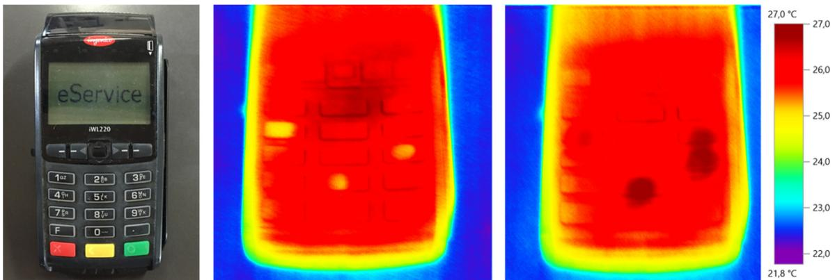
Figure 7: Attack on metal keys (orange box– keys covered with hair spray, red box – keys covered with nail polish), t. 5 s.
