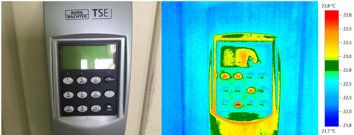
Figure 4: Attack on a combination door lock (no protective film), time: 5 seconds, PIN:1268.
