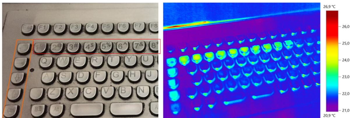
Figure 6: Attack on metal keys (orange box– keys covered with hair spray, red box – keys covered with nail polish), t. 5 s.
