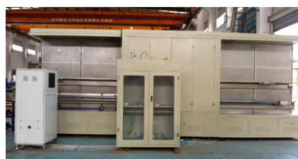
Figure 12: The prototype of the continuous diffusion furnace.
