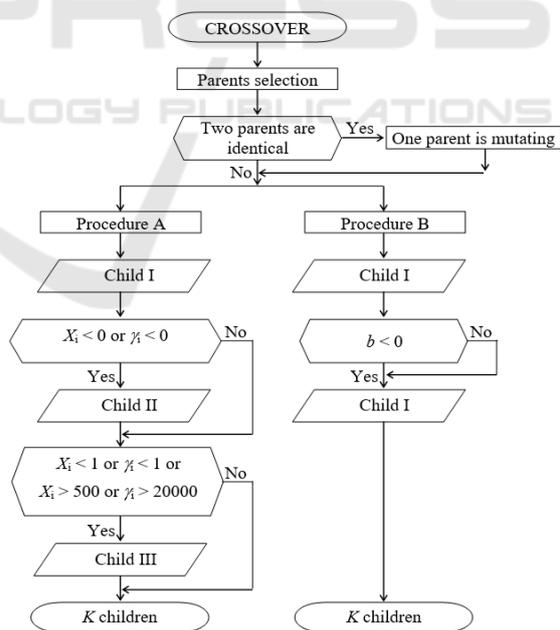
Figure 4: Crossover operator procedure.
