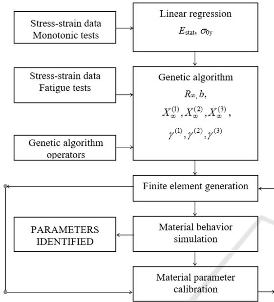
Figure 1: Parameter identification system.
