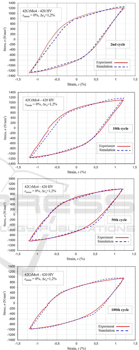
Figure 7: Stress – Strain relationships for 2<sup>nd</sup>, 10<sup>th</sup>, 50<sup>th</sup> and 100<sup>th</sup> loading cycle.
