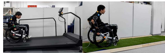
Figure 7: Left; Situation of the experiments on a slope which set the inclination to 3.4[deg] in accordance with the barrier-free law of Japan. Right; Situation of the experiments on a lawn way simulated the irregular ground.
