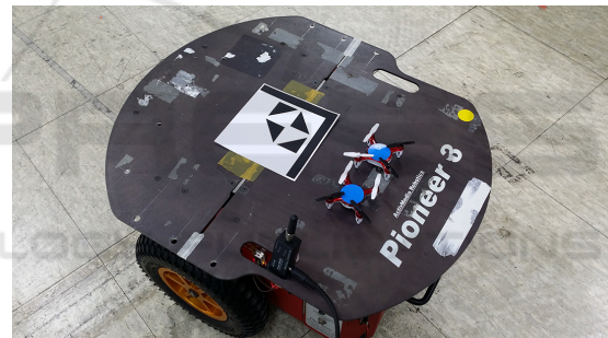
Figure 1: One Pioneer robot as the CR and two X12s as the UAVs. The CR and the UAVs can be recognized and located by using the artificial landmarks.
