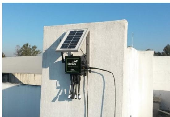
Figure 7: A sensor node located at the roof of the department building.
