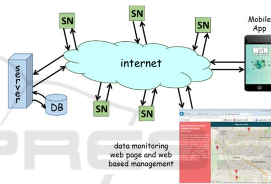
Figure 2: Elements of the wireless sensor network system.
