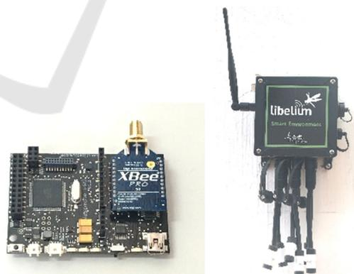
Figure 3: The Wasmote OEM version, left, and the Plug&Sense! Version, right.
