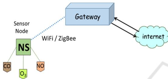
Figure 4: Communication between server and nodes through a Gateway.
