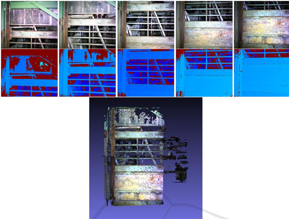
Figure 5: RGB images (upper row), depth images (second row) and reconstructed 3D model (last row).
