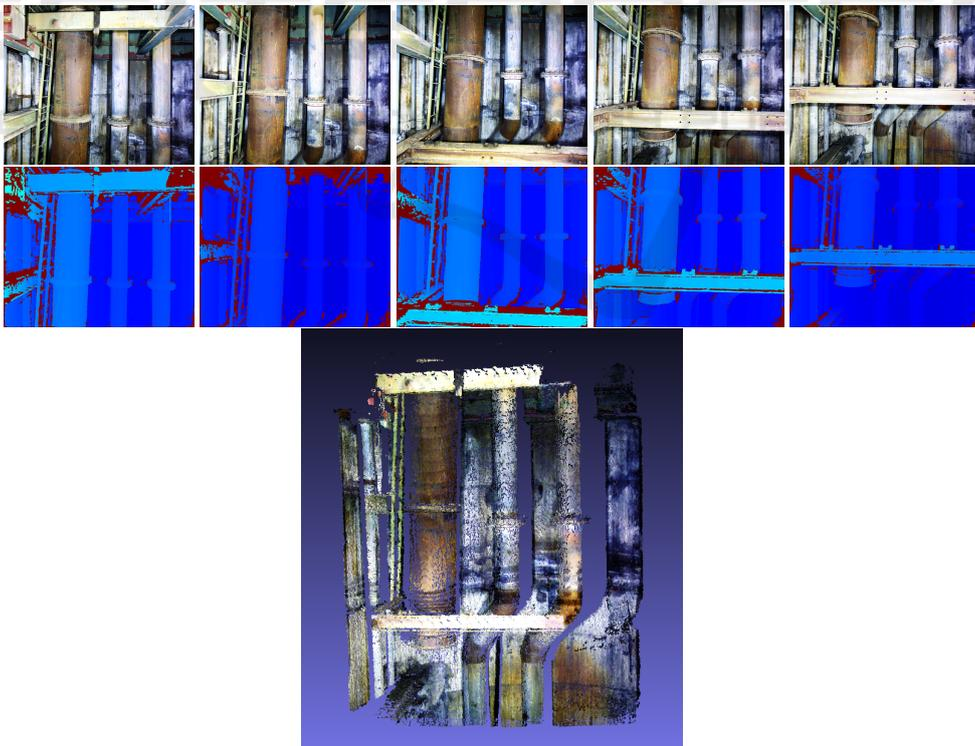
Figure 6: RGB images (upper row), depth images (second row) and reconstructed 3D model (last row).
