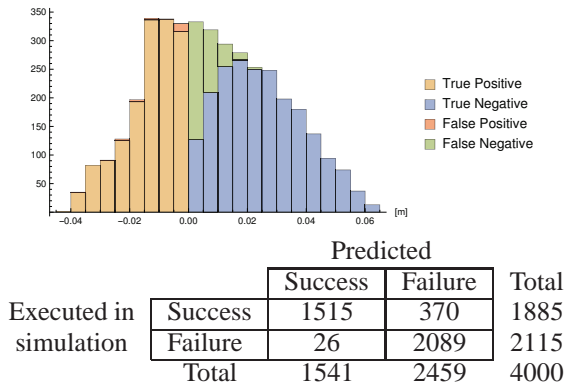
Figure 5: Histogram and confusion matrix for the 3D positional errors based on 12 lattice vectors for the grasping subtask.
