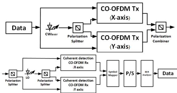
Figure 6: Conceptual diagram for PDM-CO-OFDM system.
