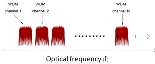
Figure 2: The optical spectrum for N wavelength-division-multiplexed CO-OFDM channels.
