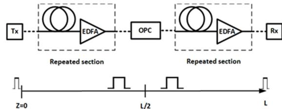
Figure 4: Long-distance transmission system employing midway optical phase conjugation (OPC).
