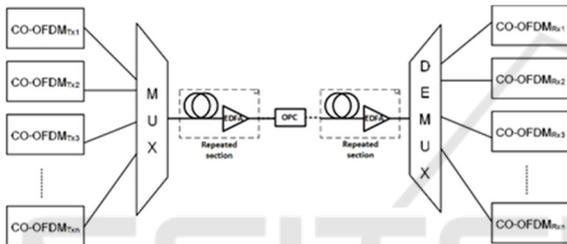
Figure 1: Configuration of Long-distance CO-OFDM transmission system employing midway OPC.
