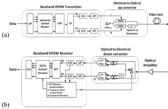
Figure 5: Conceptual diagram for complete CO-OFDM system (a) Tx, and (b) Rx.
