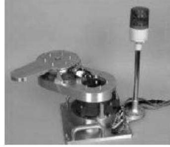
Figure 1: Two-Link Manipulator(SR-402DDII).
