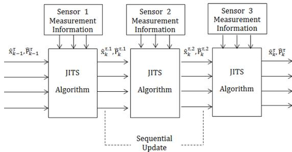
Figure 1: Sequential implementation of JITS algorithm.
