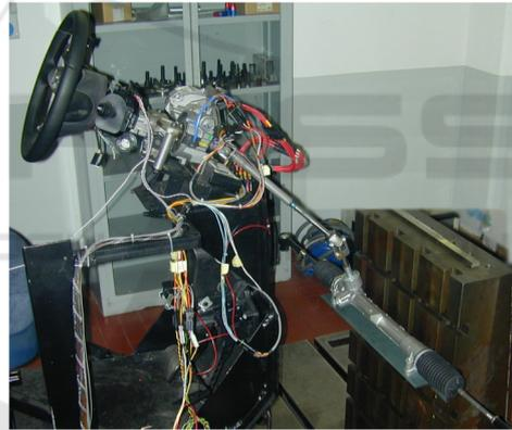
Figure 9: FCA Innovation Technical Center EPS test bench.
