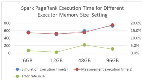
Figure 11: Spark executor memory scaling.
