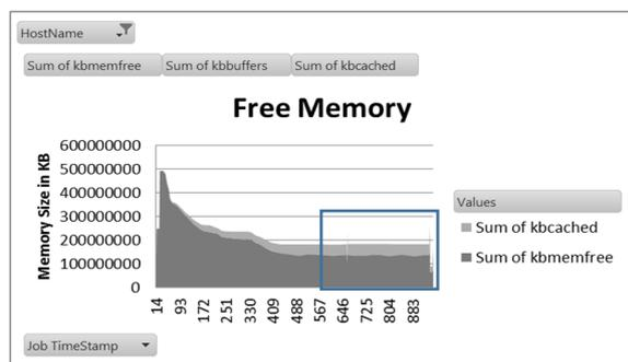
Figure 14: OS memory utilization for 45GB reserved system memory case.
