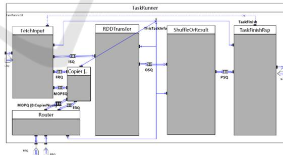
Figure 2: Middle abstraction level model of the Spark task executor.
