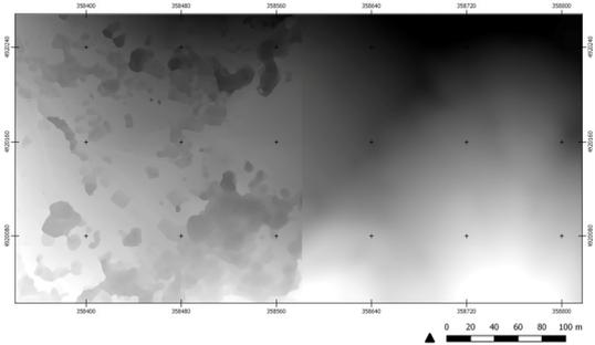
Figure 9: Comparison between the DSM generated from UAV image processing and the final DEM obtained from GIS raster analysis and filtering.
