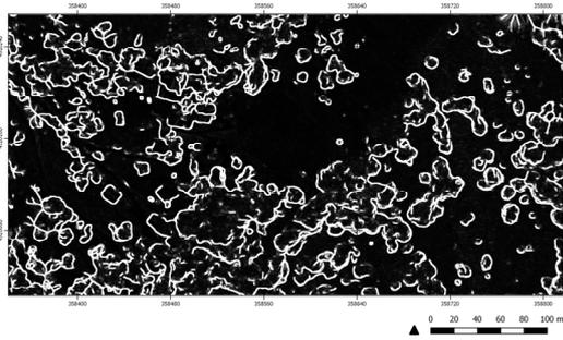
Figure 5: Applying the Terrain Ruggedness Index algorithm to de DSM: best-input value 0.05. Reclassification of the raster with binary values (0-1) to perform buffer analysis on a unique value.
