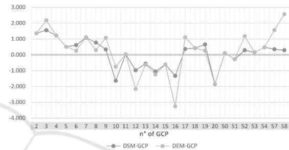
Figure 10: Residuals of DSM/DEM from GCP. The elaborated DEM, differs from DSM mainly on rich vegetation and built-up areas.
