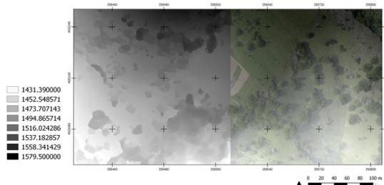
Figure 2: The DSM of the test area, compared with the orthoimage from the drone flight: it is distinct the assorted presence of vegetation cover in a very slope terrain.
