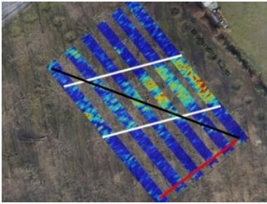
Figure 7: Superimposition of time-slice at 1.2 m of depth on orthophoto, with main anomalies derived from geophysical prospections highlighted.
