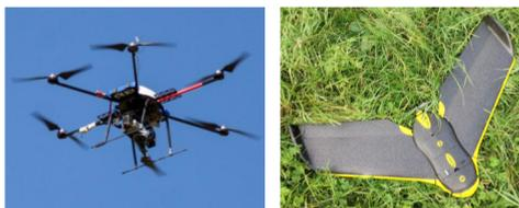
Figure 1: Two example of unmanned vehicles, the ones used in the further test: hexacopter by Mikrokopter and Ebee by Sensfly.
