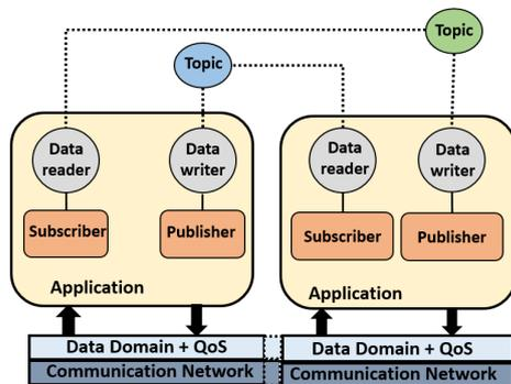
Figure 1: DDS architecture and components.
