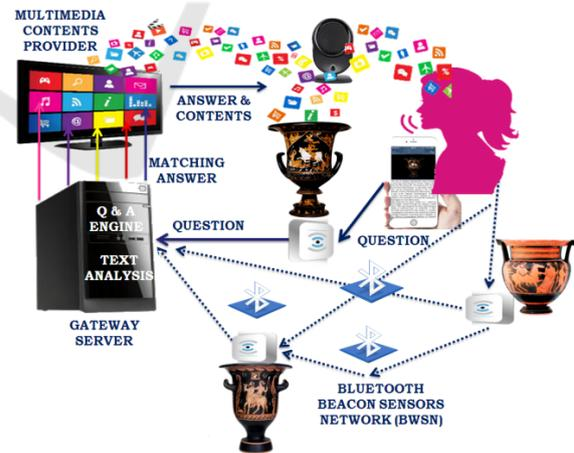
Figure 3: Service System Architecture.
