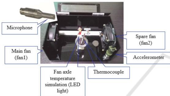
Figure 1: Simulation fixture of ATS.
