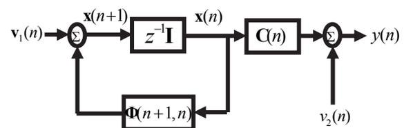
Figure 2: Block diagram of Adaptive Kalman filtering.
