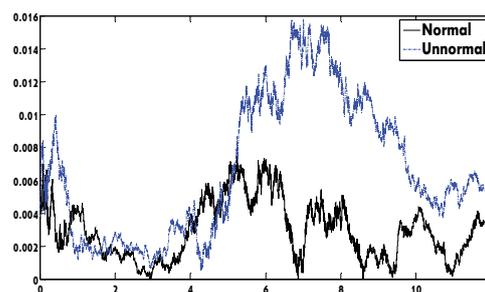
Figure 10: Adaptive Kalman filtering algorithm by using acoustic energy (the dotted line represents a failure condition while the solid line represents a normal condition).
