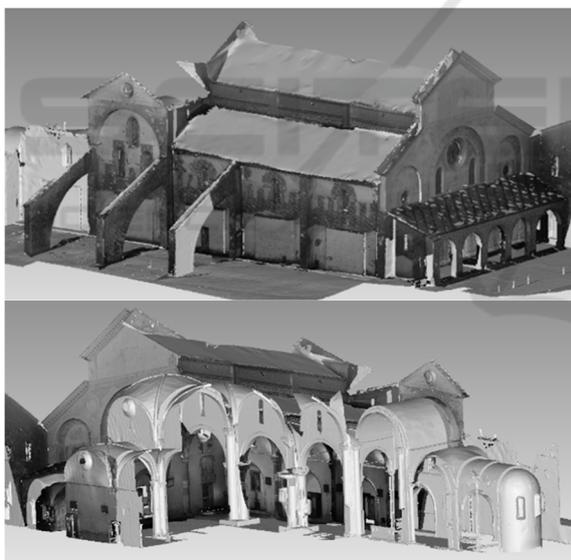
Figure 5: Views of the 3D model (textured mesh) of the Staffarda abbey church, processed using LIDAR acquisitions integrated with photogrammetric data acquired from UAV (Unmanned Aerial Vehicle) (Bastonero et al., 2014).
