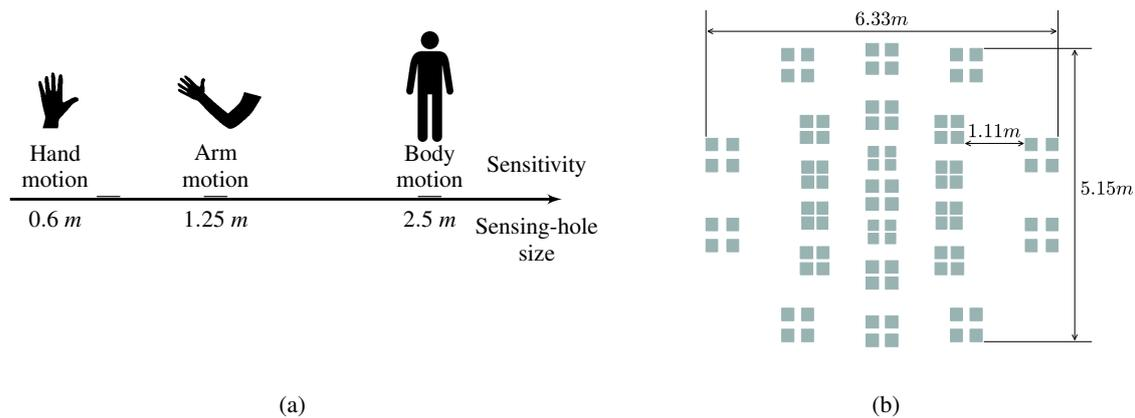
Figure 1: (a) The relation between the size of sensing-holes and motion sensitivity. (b) 2D view of a PIR Field-of-View. Solid rectangles represent detection zones.
