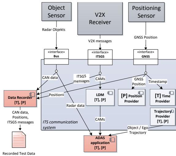
Figure 1: Software Architecture of the Evaluation System.
