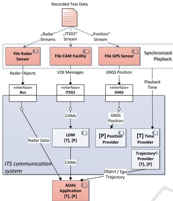
Figure 4: Synchronized information flow within the playback architecture used as offline evaluation environment.
