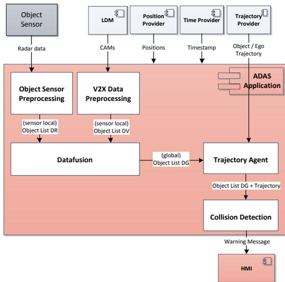
Figure 2: Information processing chain for an ADAS.
