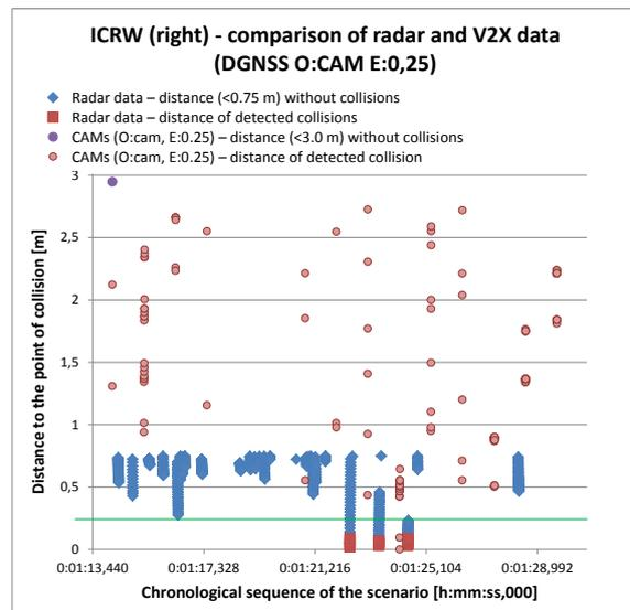
Figure 5: Comparison of radar and V2X based ADAS.
