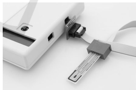
Figure 1: The potentiostat used in the research and the screen printed electrodes.
