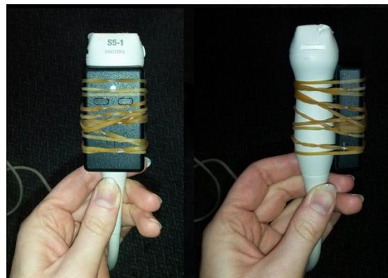
Figure 1: The inertial measurement unit sensor and the ultrasound probe.
