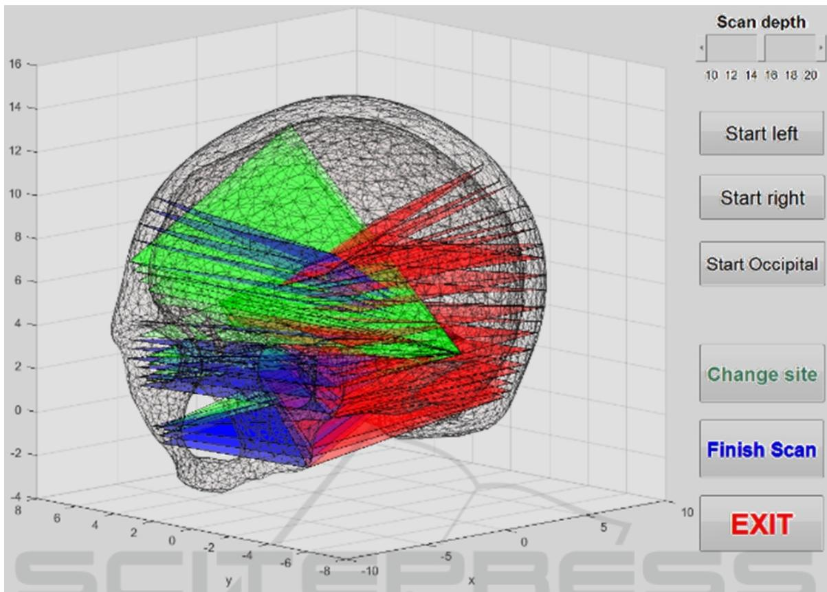
Figure 3: A screenshot of the 3D head model display program showing where scans have been performed from the different acoustic windows (red for the patient's right temporal window, green for their left temporal window and blue for the occipital window).
