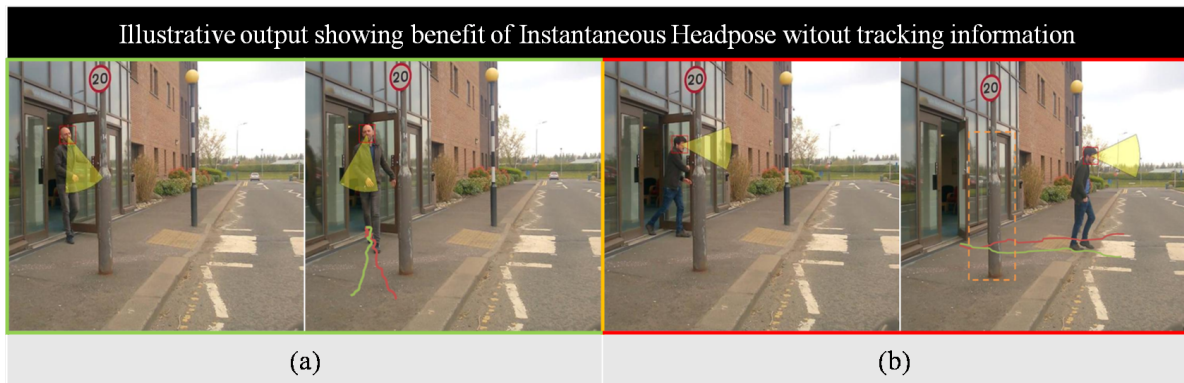
Figure 4: The benefit of headpose as a prior is clearly illustrated when no prior tracking information is available. The Kalman filter output is shown in red and the intentional tracker output is shown in green. We initialize the tracker with very few frames and let the trackers evolve without further detection. (a) The person does not cross the road and his headpose at the instant of exiting the door is very indicative. (b) Similarly for people who want to cross the road, the head pose information is again very indicative of their intention. There is a region of occlusion that is shown in orange. The trajectories qualitatively show the benefit of the intentional tracker.
