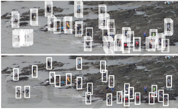
Figure 7: Detection after the sliding window method (top) and after merging positive rectangles (bottom).
