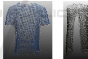
Figure 4: Left to right: aligned shirt and trouser point clouds after manually removing several outliers.
