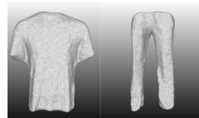
Figure 5: Left to right: reconstructed shirt and trouser mesh after using Poisson surface reconstruction.
