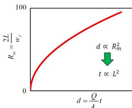
Figure 15: Almost parabolic relationship between the mixing ratio  $R_m$  and the distance  $d$  from the junction point. If the curve is parabolic,  $t$  is proportional to  $L^2$ .
