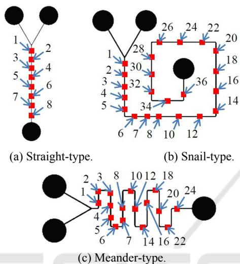
Figure 8: Points where the mixing ratio  $R_m$  was evaluated.
