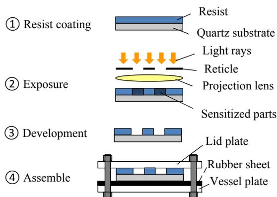
Figure 1: Fabrication method of micro-mixer.
