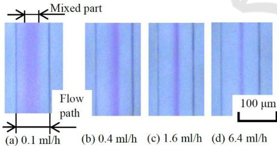
Figure 13: Visual differences of mixed flows observed at point 3 of the snail-type mixer.
