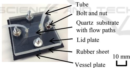
Figure 5: Assembled micro-mixer.
