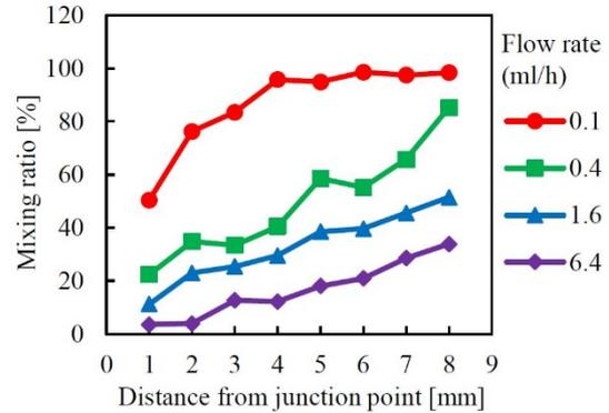
Figure 14: Mixing ratio of straight-type micro-mixer with a flow-path width of 50 μm.
