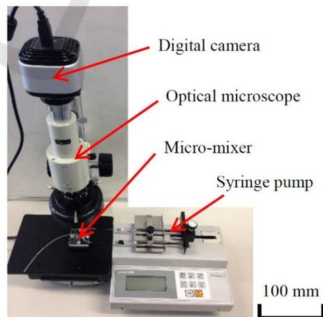
Figure 6: Set up for injecting liquids in the micro-mixer and in situ observation system.
