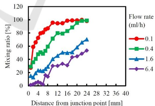
Figure 11: Mixing ratio of meander-type micro-mixer with a flow-path width of 100  $\mu\text{m}$ .
