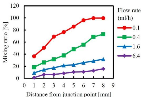
Figure 9: Mixing ratio of straight-type micro-mixer with a flow-path width of 100  $\mu\text{m}$ .
