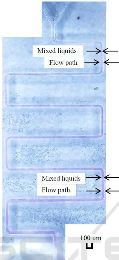
Figure 12: Panoramic photograph of meander-type mixer. It is clearly observed that the flow width of mixed liquids increases gradually from the junction point to the outlet.
