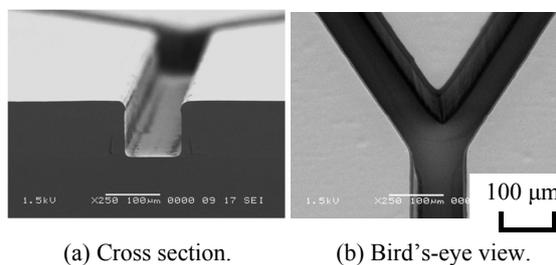
Figure 3: Profiles of flow-path patterns.
