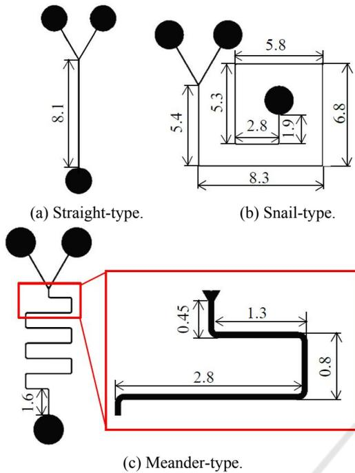
Figure 4: Shapes and sizes of fabricated micro-mixers.
