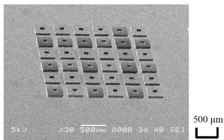
Figure 9: Dispersively arrayed 300-μm square patterns with 100-μm square hollow cells.
