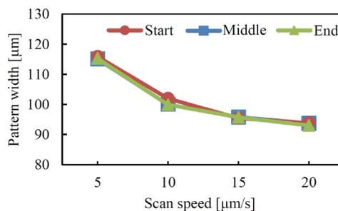
Figure 11: Pattern width control by adjusting the scan speed.
