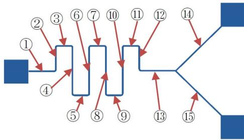
Figure 13: Points selected for measuring pattern widths.
