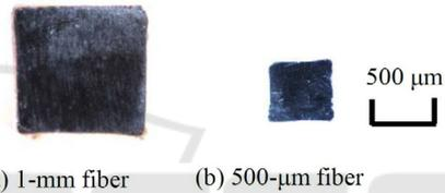
Figure 15: Half-size squared optical fiber with a cross section profile similar to that of current size fiber.
