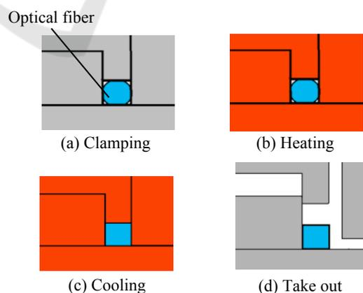
Figure 2: Method used for deforming optical fiber ends to square shapes.
