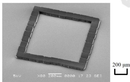
Figure 8: Chamber pattern with 800-μm square chamber and 100-μm wide fence.
