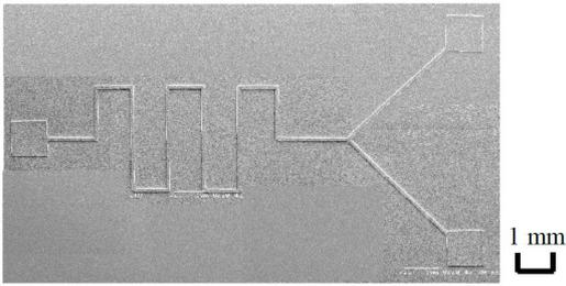
Figure 12: Micro-fluidic device pattern.
