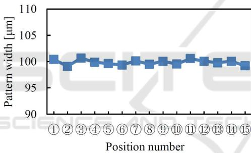
Figure 14: Width homogeneity of fabricated micro-fluidic device patterns.
