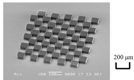
Figure 6: Printed checker patterns usable as a cell array.
