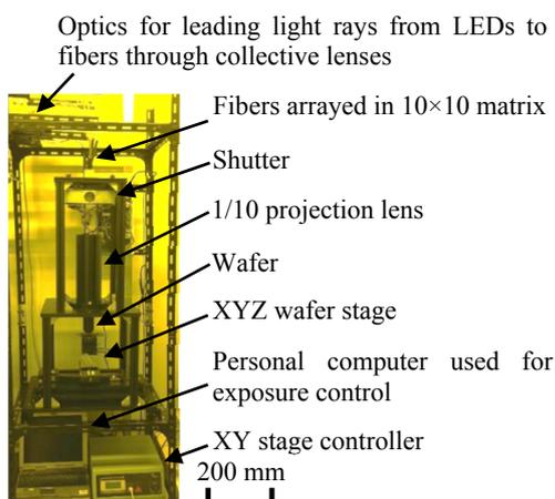
Figure 1: Exposure system used for the research.
