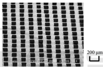
Figure 10: Arrayed 100-μm square pillars. If patterns were replicated to PDMS using soft lithography, a cell array would be obtained.
