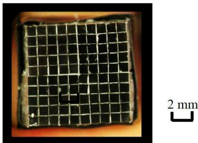
Figure 5: Fibers arrayed in a  $10 \times 10$  matrix and fixed to the exposure system.
