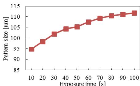
Figure 7: Pattern size controllability by adjusting the exposure time.
