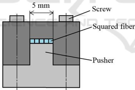
Figure 4: Bundling instrument used for aligning and bonding squared 5 fibers, and piling them.
