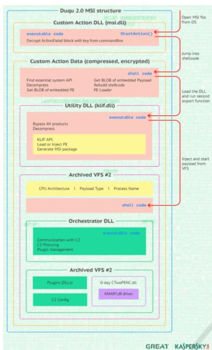
Figure 3: Kaspersky's breakdown of Duqu's MSI structure. (Kaspersky, 2015).
