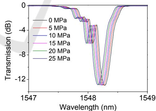
Figure 5: Evolution of the transmission spectra of PS-FBG under different pressures.
