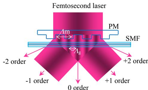
Figure 1: Schematic diagram of the PS-FBG inscription by femtosecond laser.
