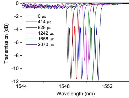
Figure 7: Evolution of the transmission spectra under different strains.
