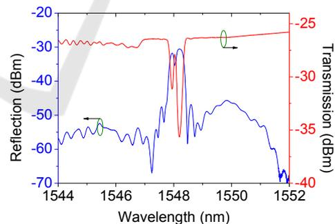
Figure 2: Reflection and transmission spectra of the PS-FBG inscribed by femtosecond laser.
