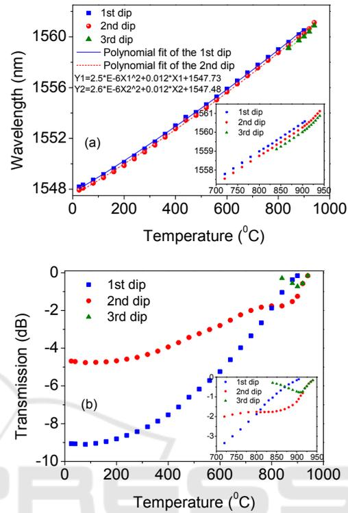
Figure 4: Change of the (a) central wavelengths and (b) transmission losses for two dips with the temperature.
