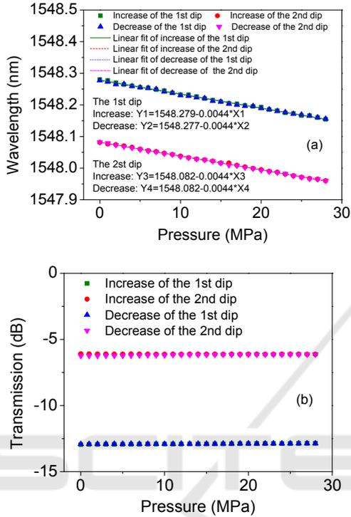
Figure 6: Changes of the (a) central wavelengths and (b) transmission losses for two dips under different pressures.
