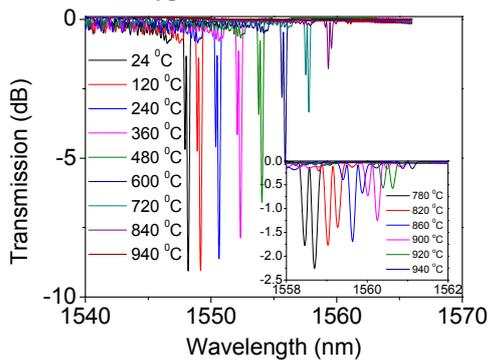
Figure 3: Evolution of the transmission spectra of PS-FBG under different temperature.
