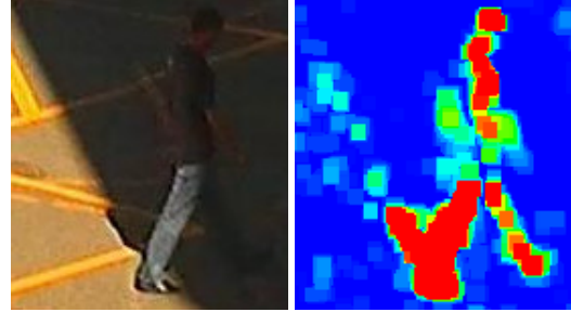
Figure 6: Reliability map using naive background subtraction. Left image: current image, right image: reliability map from naive background subtraction.
