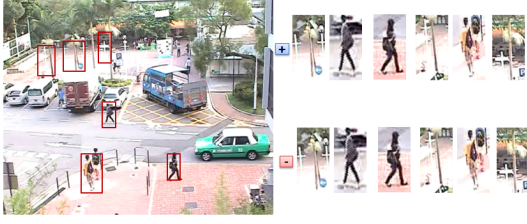
Figure 4: Illustration of the prediction step result: Detections provided by a generic detector applied on frames of the CUHK_Square dataset.
