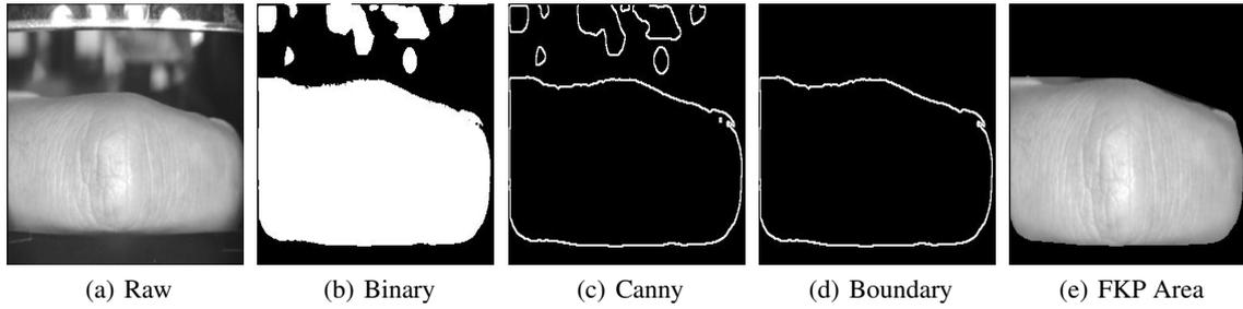
Figure 5: Steps involved in Knuckle Area Detection.
