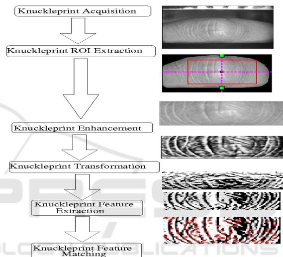
Figure 3: Overall architecture of FKP recognition system.
