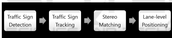
Figure 2: Flow chart of the proposed vehicle lane-level positioning system.
