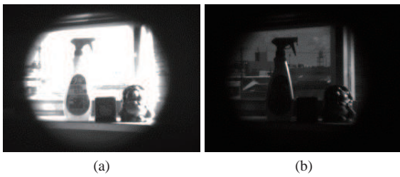
Figure 7: Observed images taken by an ordinary camera with long exposure time (a) and short exposure time (b).
