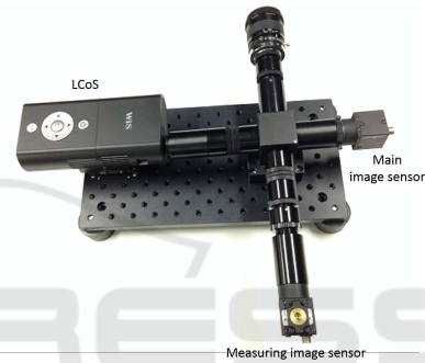
Figure 6: Variable exposure camera. It consists of an LCoS device and two image sensors.
