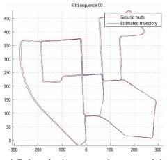
Figure 4: Estimated trajectory vs. trajectory recorded using GPS/IMU for KITTI sequence 00, scale in [m].
