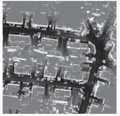
Figure 1: Small section of an occupancy grid map with cell size 12.5x12.5cm.
