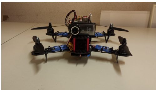
Figure 11: The UAV where we did our experiment with. X-Bird 250 equipped with an Odroid XU3 processing board.
