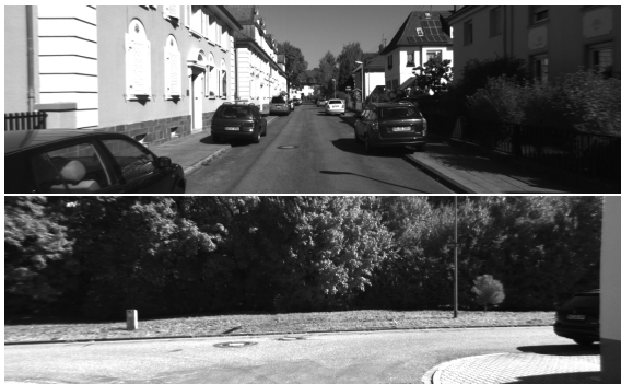
Figure 9: Images of the KITTI visual odometry dataset (sequence 07). In this sequence, there are some lines detectable in some parts (e.g. in top image). In these parts, the detected lines are beneficial for the VO algorithm. However, in some images there exist no lines (e.g. image bottom) and our algorithm also depends on the detected feature points.
