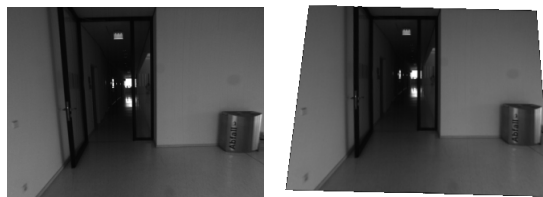
Figure 2: Image alignment according to the gravity direction. Left : An unaligned image from a forwards looking camera Right : Image aligned using the IMU. As one can see, having an image aligned according to the gravity direction, straight, vertical lines in the 3D scene are mapped to straight, vertical lines in the image.
