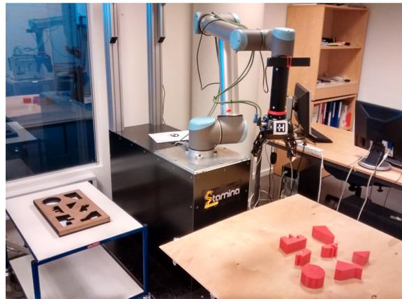
Figure 2: Complete lab setup. The 7 considered objects can be seen at the lower-right part of the picture, while the kitting box on the left.
