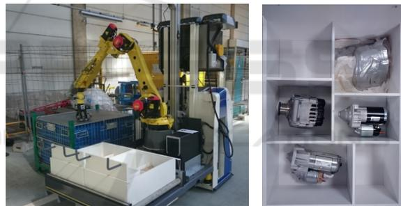
Figure 1: The STAMINA mobile robot (left) manipulating objects and filling two kitting boxes placed in the front of the robotic platform. A closeup of a kitting box structure (right).
