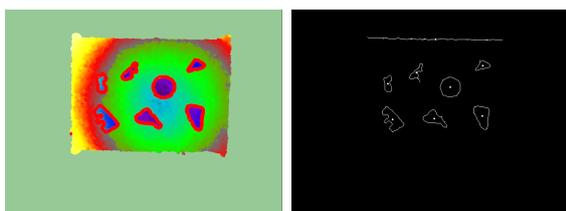
Figure 5: The filtered point cloud (left) and the filtered detected edges on the depth image (right).
