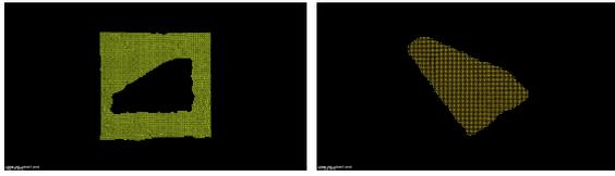
Figure 9: The box-hole (left) and the object (right) point clouds input for the ICP algorithm.
