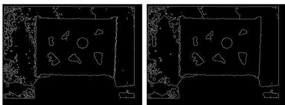
Figure 4: Edges in a typical image detected by Canny (left) and the same edges after applying dilation-erosion (right).
