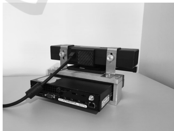
Figure 2: Sensor mounted on mini PC via clamp.
