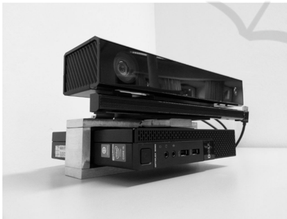
Figure 3: Fixation of Kinect v2 on top of mini PC.
