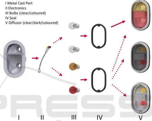
Figure 2: Assembly states of tail lights.(Ganji et al., 2010).
