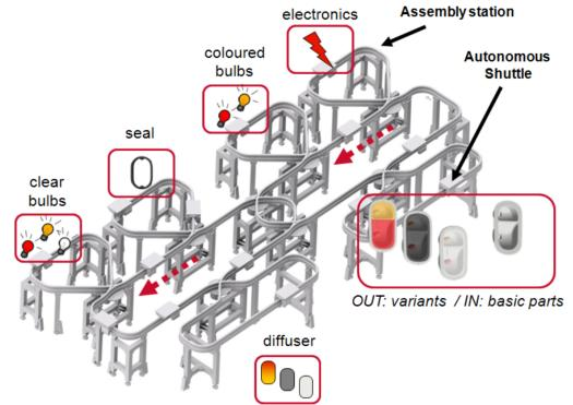
Figure 1: Assembly scenario for tail-lights (Morales Kluge et al., 2010).
