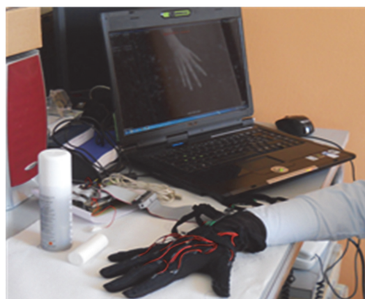
Figure 1: The sensory glove prototype and the experimental materials.
